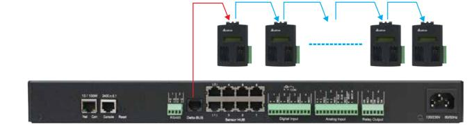
▲ Connecting EnviroProbes with EnviroStation can expand the scope of the monitored area.
