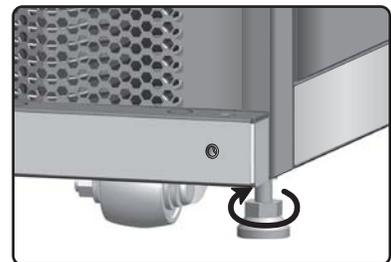
(Figure 3-6: Rotate Each Leveler Clockwise)
