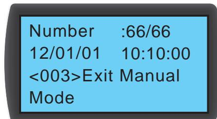
On this screen, No. means the current event / total events. A maximum of 3000 events can be recorded in the log. Press ▲ ▼ to switch between events, which are sorted in chronological order, that is, the No. grows with the new event. The figure in < > indicates the event code. If more than 3000 events are recorded, the oldest events will be overwritten.
