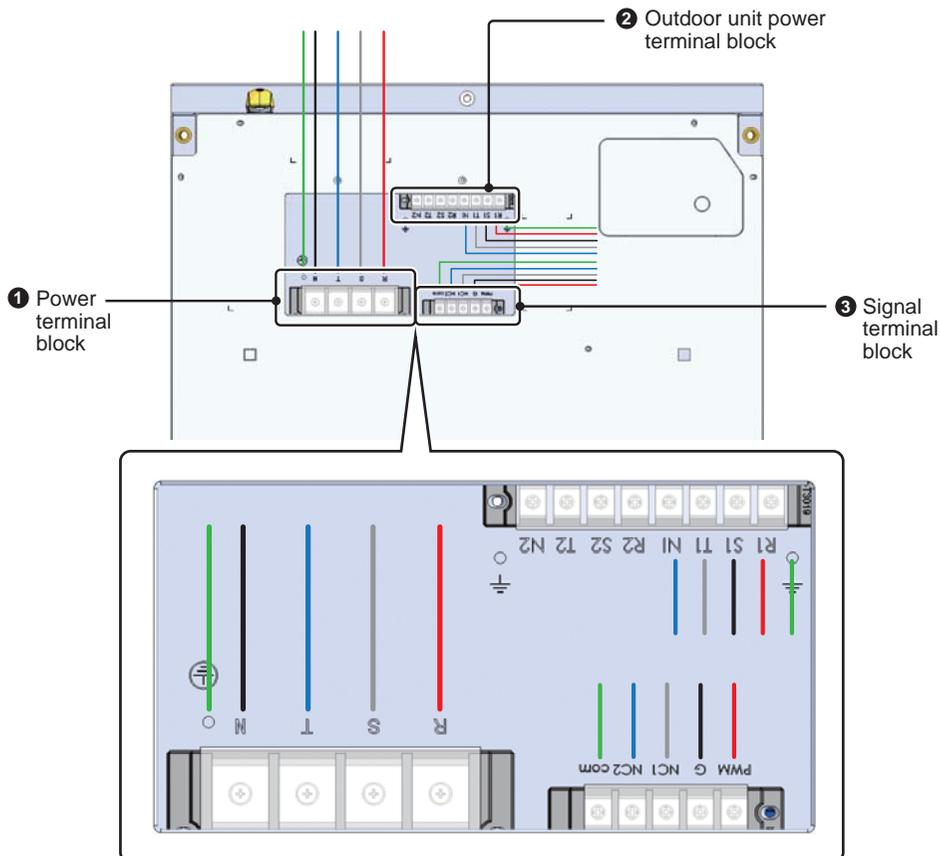
(Figure 3-17: Install the Power Cables & Signal Lines)
