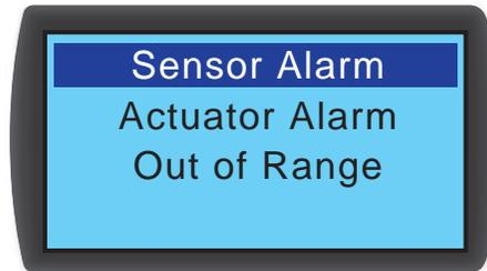
Set the 'Sensor Alarm', 'Actuator Alarm' and 'Out of Range' alarm. For the item with , it means this alarm is disabled. Press **←** at this item, use **▲ ▼** to select , and press **←** to confirm to enable this alarm.
