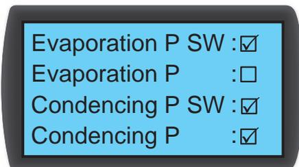
Set the alarm ON or OFF for Return Sensor, Supply Sensor, Remote Sensor 1 ~ 4, Air Sensor, Leak SEN.(leakage sensitivity), Evaporation P SW (low pressure switch), Evaporation P (evaporation pressure sensor), Condensing P SW (high pressure switch), and Condensing P (condensing pressure sensor).
