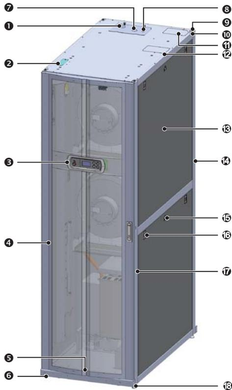
(Figure 2-3: Schematic Diagram of External Components)
