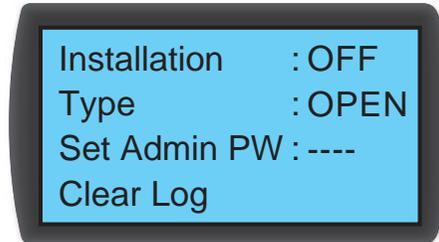
Follow your data center's cold/ hot aisle configurations to set up the system Type as **OPEN** or **CLOSE**.
