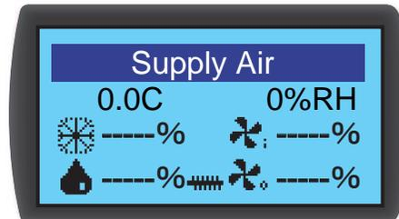
The LCD will be off during idling. Press to turn on the backlight and display the Status page. You are able to view the supply air state and output percentage of the compressor, humidifier, reheaters and indoor and outdoor fans.
