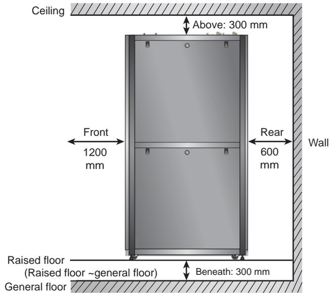
*(Figure 3-1: Clearance for Indoor Unit)*
