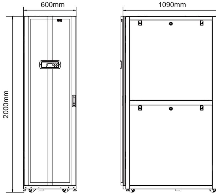
(Figure 2-1: Appearance & Dimensions of Indoor Unit)
