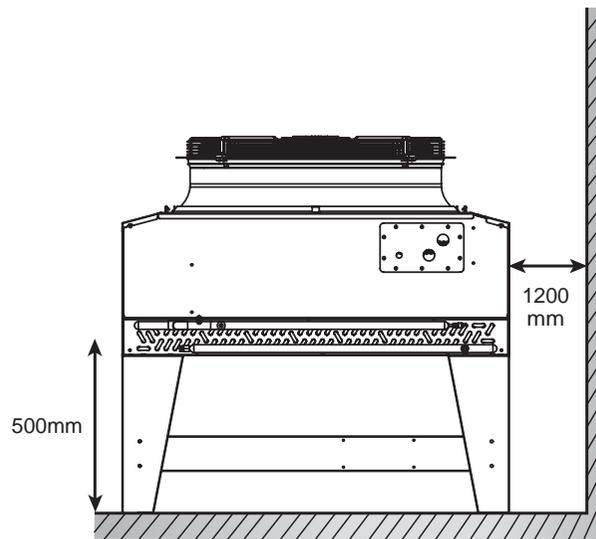
(Figure 3-2: Clearance for Outdoor Unit - Horizontal Type)
