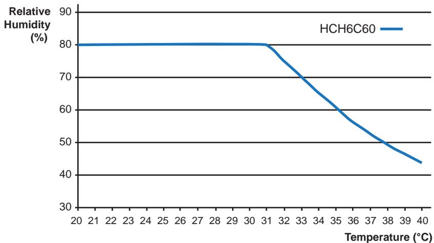
(Figure 4-2: Standard Operating Environment Conditions)
