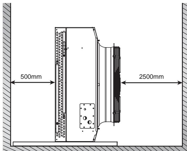
(Figure 3-3: Clearance for Outdoor Unit - Vertical Type)
