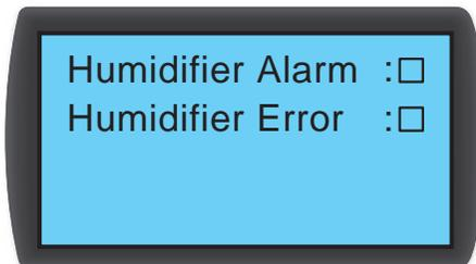
Set the alarm ON or OFF for Indoor Fan 1, Indoor Fan 2, Outdoor Fan 1, Outdoor Fan 2, Compressor Error, Heater 1 Error, Heater 2 Error, Heater Protect, Humidifier Alarm, and Humidifier Error.
