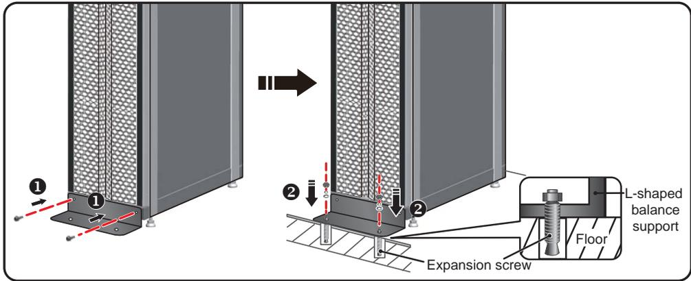
(Figure 3-8: L-shaped Balance Support Installation)
