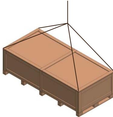
(Figure 3-5: Handling with a Hoist System)
