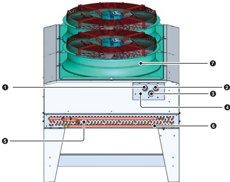
(Figure 2-7: Schematic Diagram of Main Components of Outdoor Unit)
