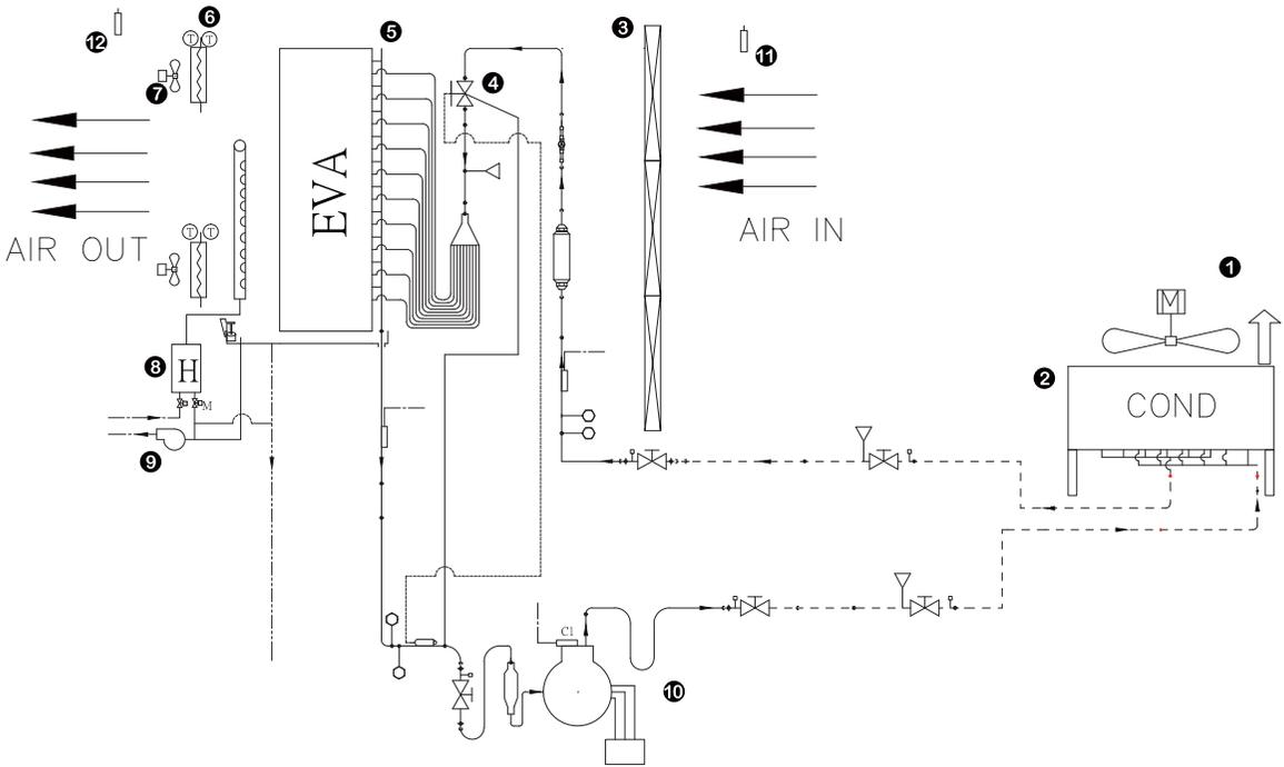
(The pipeline to be installed on site is indicated by dotted lines)
