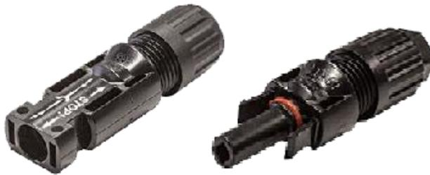
Single male/female cable coupler is compatible with MC4 connectors and is suitable with solar power cable H1Z2Z2-K with cross section 2.5mm<sup>2</sup>; 4mm<sup>2</sup> and 6mm<sup>2</sup>.
